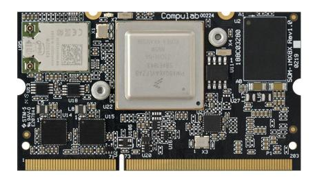
CL-SOM-iMX8X is a tiny Computer-on-Module (CoM) built around i.MX8 Quad X Plus. Built with a high-level integration to support graphics, video, image processing, audio and voice functions, it is ideal for safety-certificable and efficient performance requirements and applications such as industrial automation, HMI, industrial control, robotics, building control, automotive cluster, display audio infotainment, and telematics applications.
